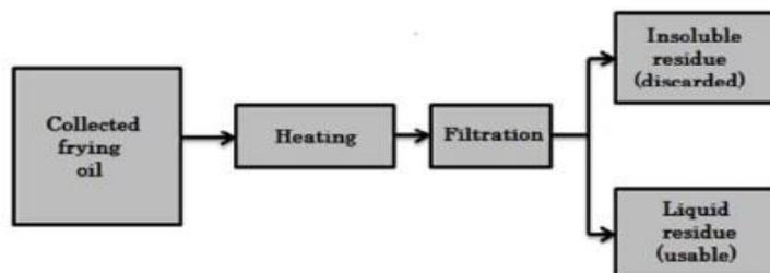
Fig.1. Pre-treatment process of cooking oil
