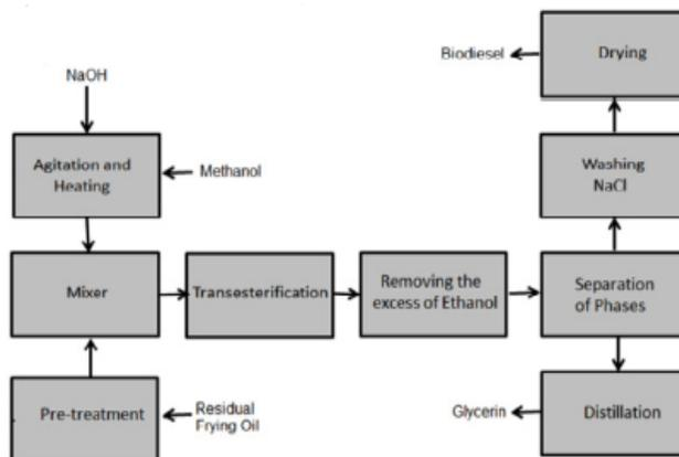
*Fig. 2. Process of Transesterification*
